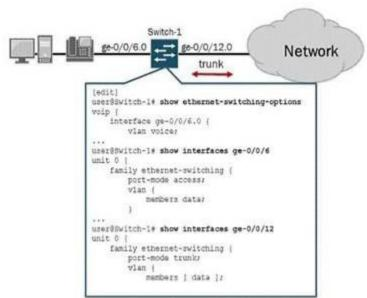
The phone connected to switch-1 in the exhibit cannot communicate with the rest of the network. How do you solve this problem?
