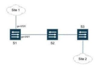
In the exhibit, switches S1, S2, and S3 have Q-in-Q tunneling configured between Site 1 and Site 2.
