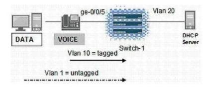
You are attaching into an EX Series switch-1a legacy IP phone that does not support LLDP-MED, but does allow configuration using DHCP, as shown in the exhibit.
