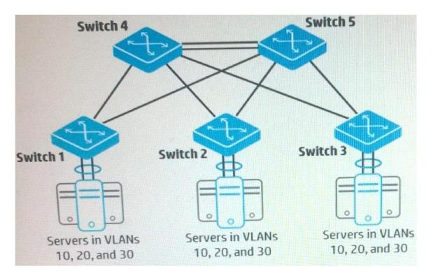
The switches shown in the exhibit form a TRILL region. What helps to load balance traffic across the .inks between these switches?
