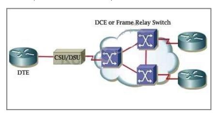
A modem modulates outgoing digital signals from a computer or other digital device to analog signals for a conventional copper twisted pair telephone line and demodulates the incoming analog signal and converts it to a digital signal for the digital device. A CSU/DSU is used between two digital lines -
