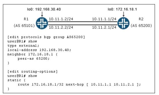
Referring to the exhibit, what must be added to the existing configuration to ensure that per-prefix load balancing occurs?
