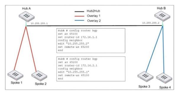
An administrator must configure an ADVPN using IBGP and EBGP to connect overlay network 1 with 2.
